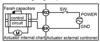
·When SW is CLOSED, the valve OPEN, the actuator automatically power off after in place.
